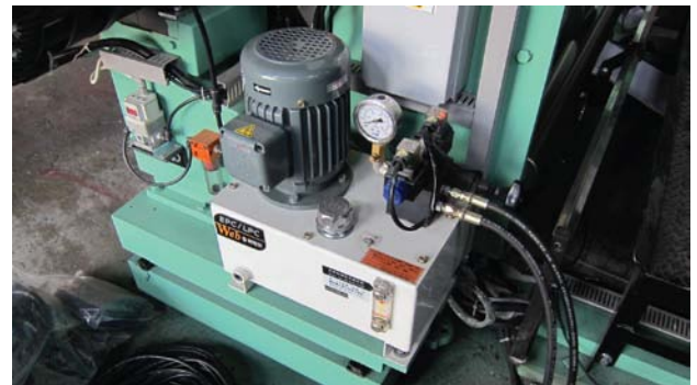
Hydraulic Actuator AO-2GH is used on a Laminator for Unwinding
