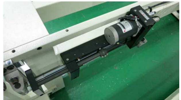
Electrical Actuator BA is used on a Rewinding Machine for Rewinding
