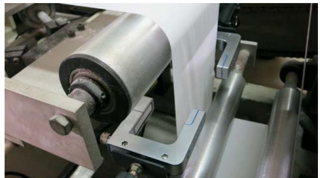
Ultrasonic Wideband Sensors DU-2N are used on a Tissue Machine for Center Position Control
