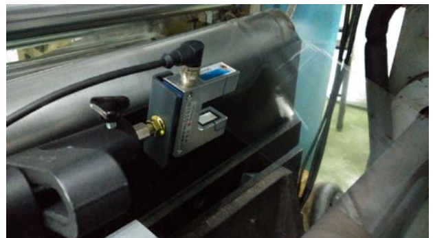
Ultrasonic Wideband Sensor DU-1N is used on a Rewinding Machine for Edge Position Control
