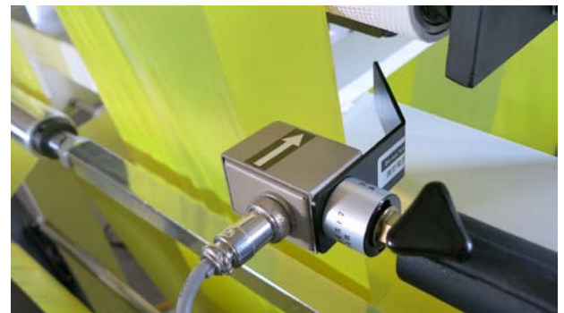
Photoelectric Sensor DT-6 is used on a Bag Making Machine
