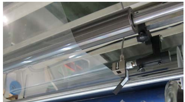
Photoelectric Sensor DT-6 is used on Clear Film
